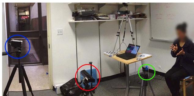
Figure 1. Experimental setup: In red on the bottom is the Kinect, recording body activity of our participant. In green, bottom-right is the Leap Motion device, recording hand activity. In blue on the left, the HD video camera.
